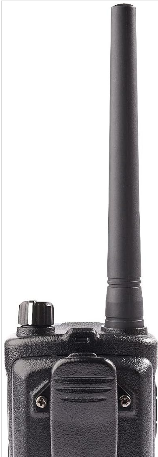
Figure 3: Side view of the Dynascan RD-5, showing the attached belt clip and side buttons.
