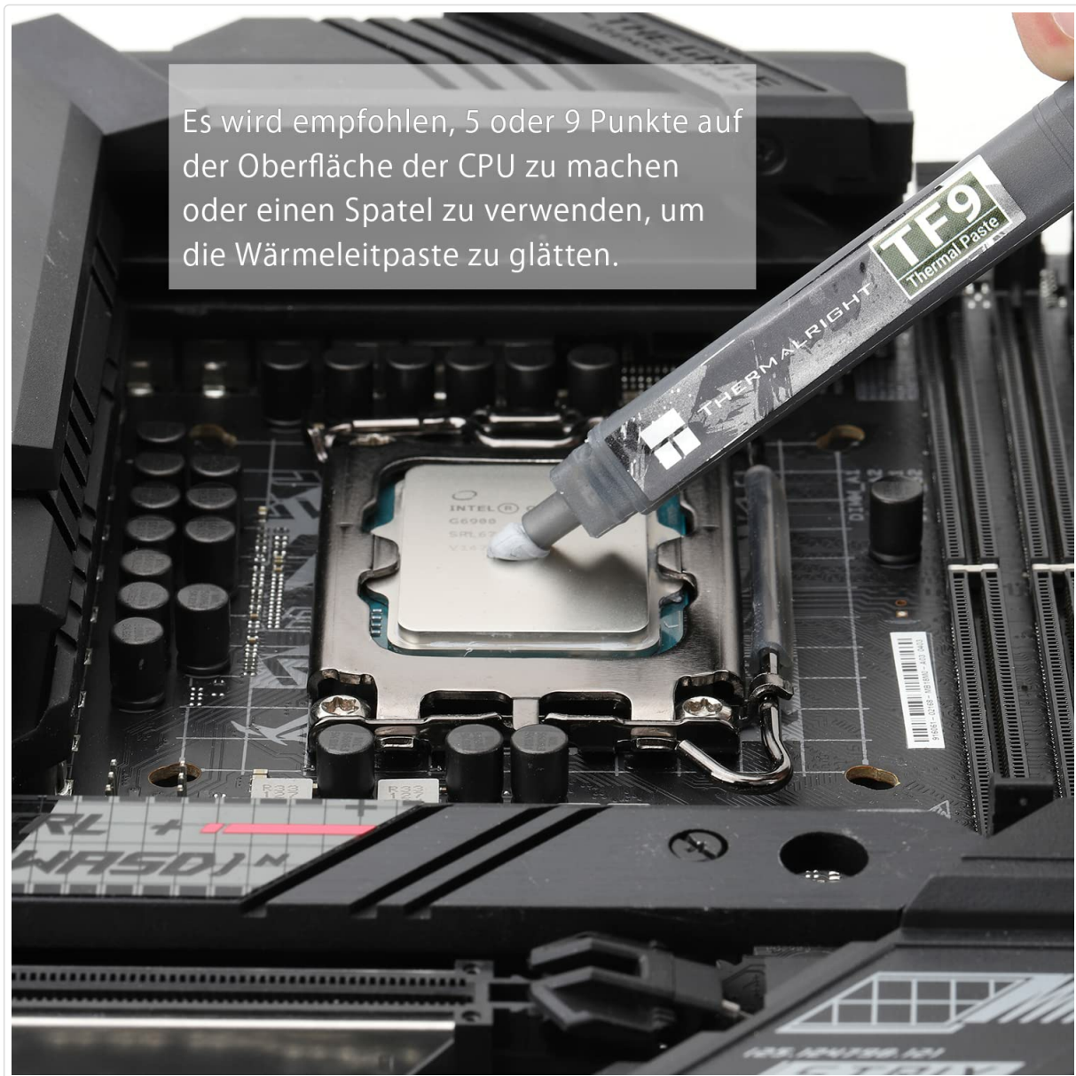
Image: Thermal paste applied in a dot pattern on a CPU, demonstrating a common application technique.
