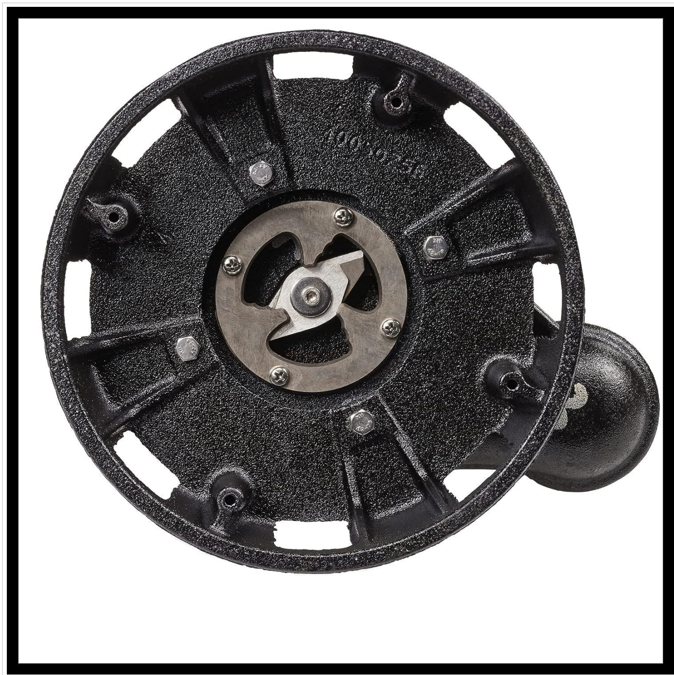
Figure 3.4: View of the integrated cutting mechanism located at the base of the pump. This mechanism is designed to shred solid particles up to 35 mm in diameter, preventing blockages.
