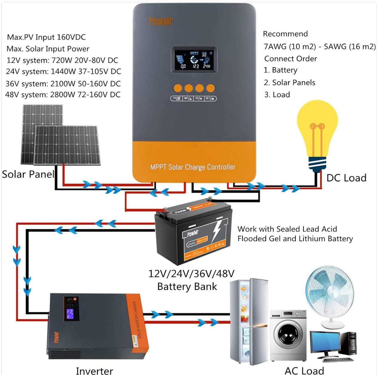
Figure 2: Typical system connection diagram for the solar charge controller, showing connections to solar panels, battery bank, inverter, and DC/AC loads.
