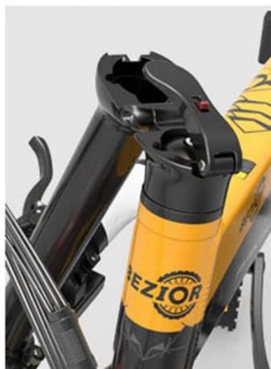
2: folding the handlebars
