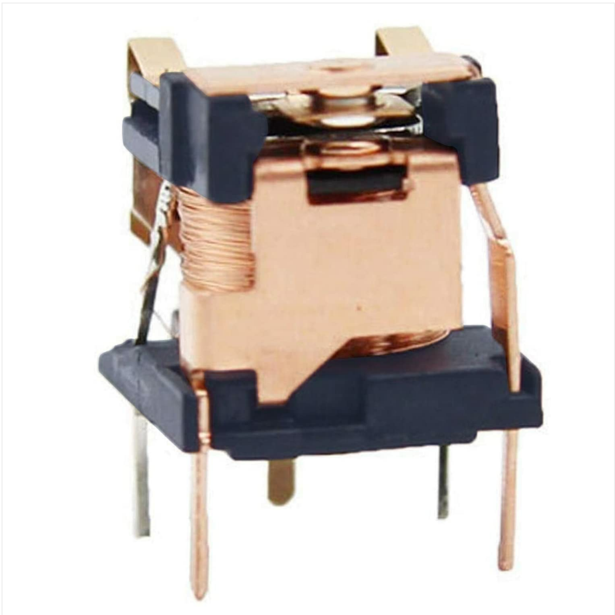
Figure 4.2: Internal structure of an electromagnetic relay, highlighting the coil and contact mechanism.
