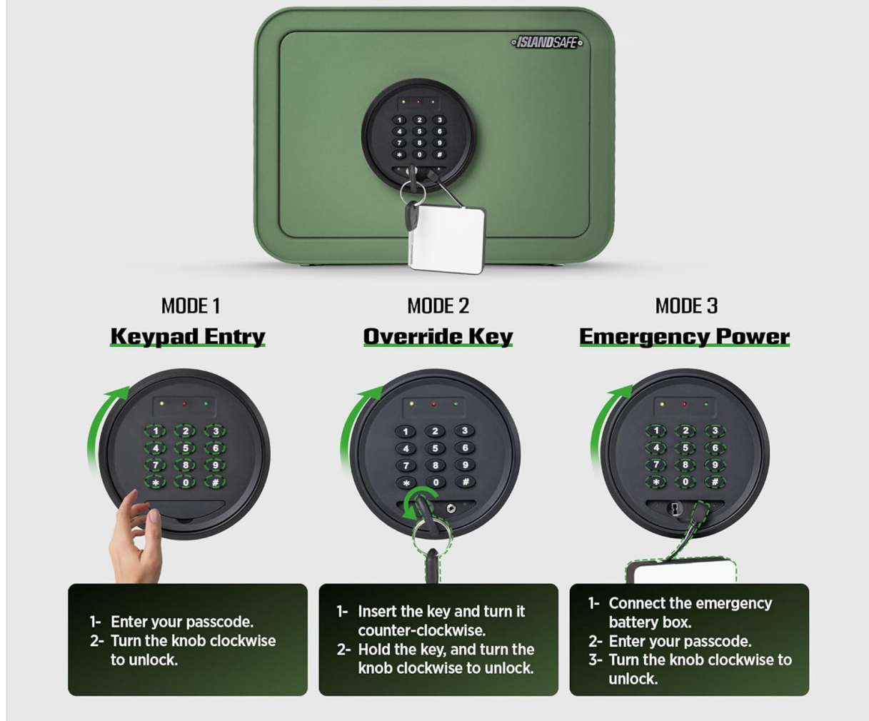
Image 6.1: An overview of the three secure access modes for the safe: Keypad Entry, Override Key, and Emergency Power.
