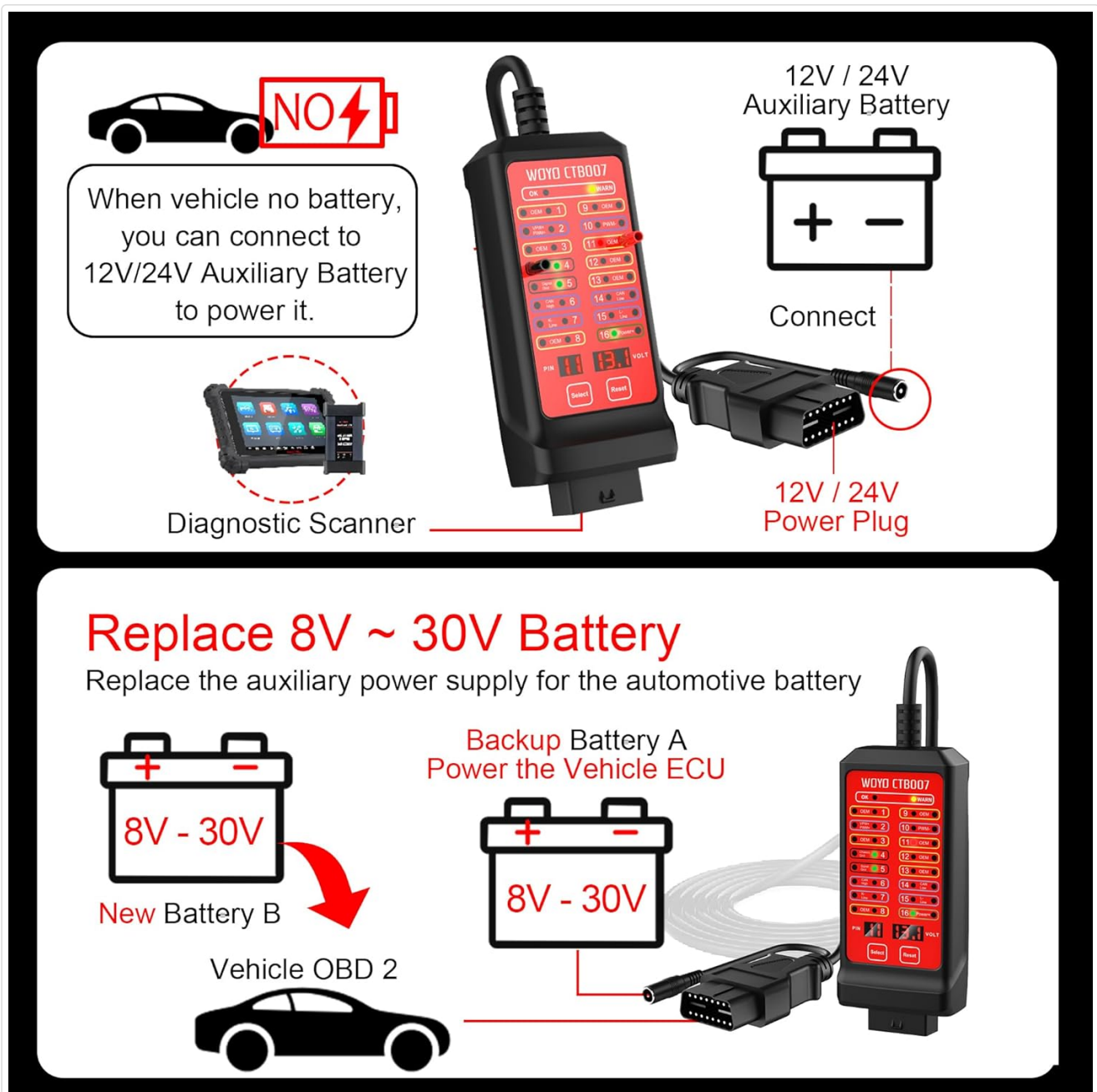
Figure 3.2: Illustration of power supply options for the CTB007. It can be powered by the vehicle's OBD2 port or an external 12V/24V auxiliary battery. It also supports maintaining ECU power during battery replacement using an external 8V-30V backup battery.
