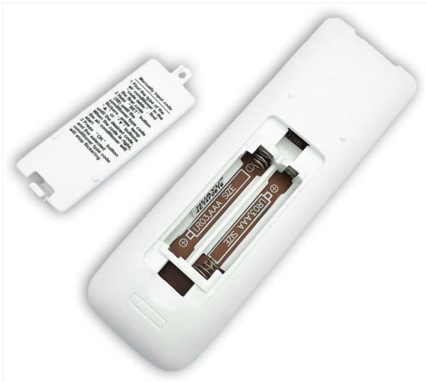
Image: Back of the remote control with the battery compartment open, illustrating where to insert two AAA batteries. Manual code input instructions are also visible on the battery cover.
