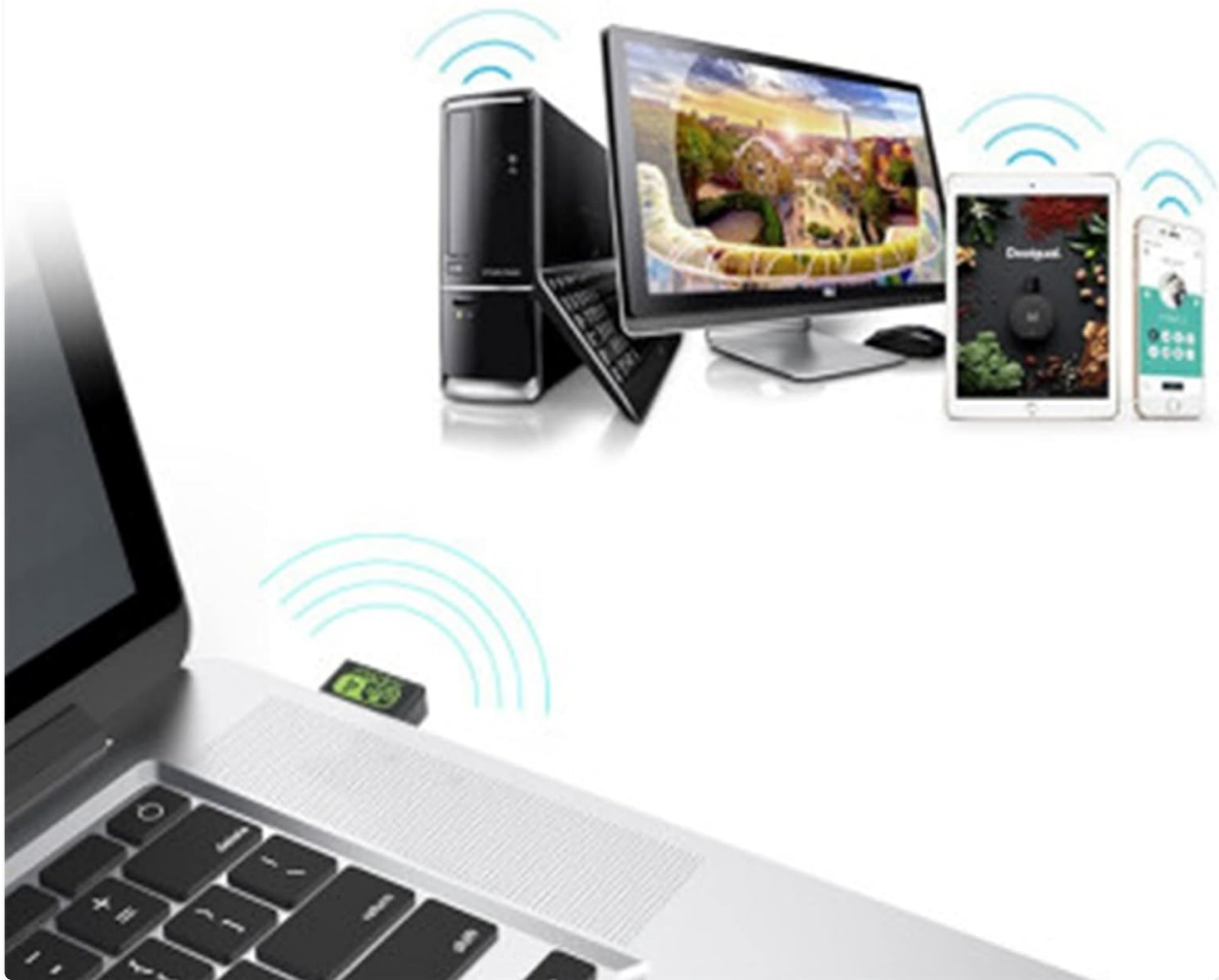
Image 5.1: Illustration of the Soft-AP Mode, where the USB WiFi adapter allows a laptop to share its internet connection with other wireless devices like a desktop computer, smartphone, and tablet.
