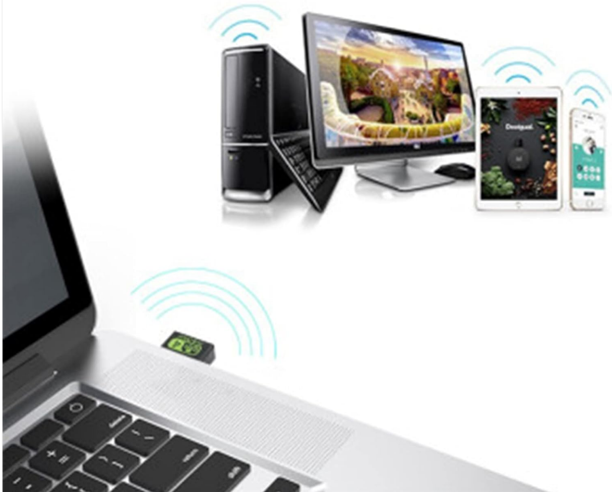
Image 5: Illustration of Soft-AP mode, where the USB WiFi adapter enables a computer to share its internet connection wirelessly.
