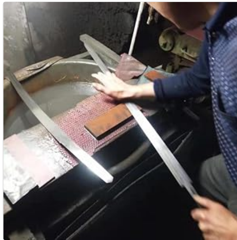
Figure 5.4: The final polishing stage, where the blade is meticulously refined to achieve its sharp edge and finish.
