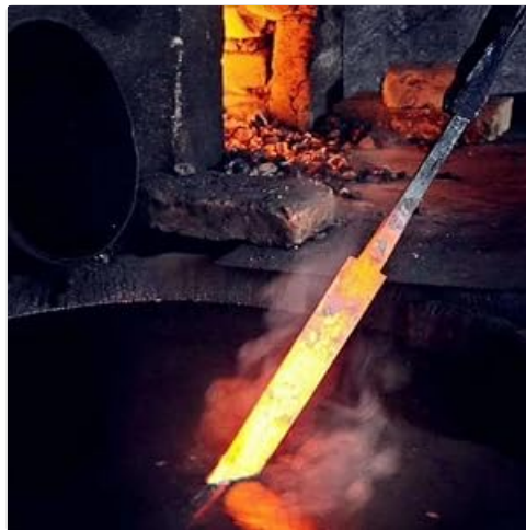
Figure 5.2: The quenching process, where the heated blade is rapidly cooled to harden the steel.
