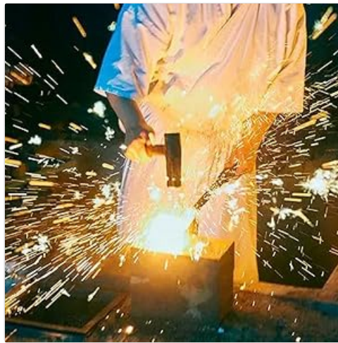
Figure 5.1: The forging process, where the steel is hammered to shape the blade.
