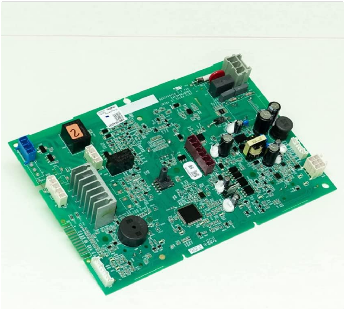
Figure 4.1: Top view of the Interface Control Board, showing various connection points for wire harnesses. Note the different colored and shaped connectors.
