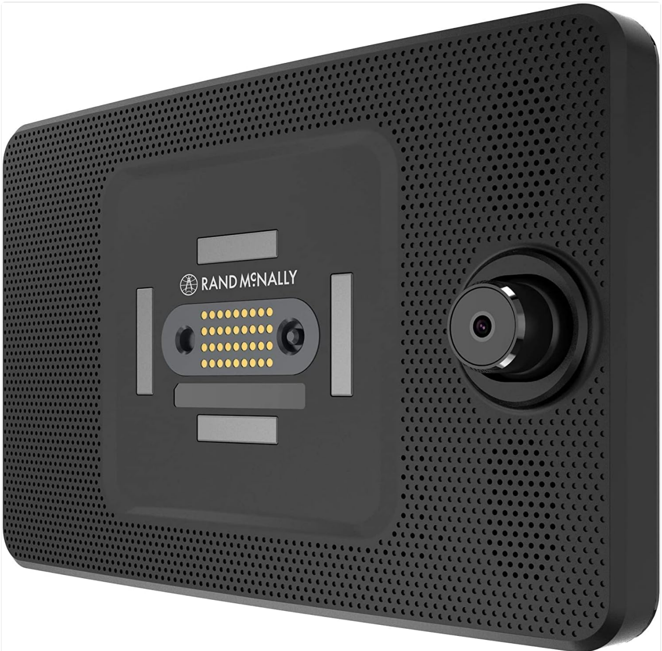
Image 3.4: Rear view of the device, displaying the magnetic mounting interface and the integrated dash camera.
