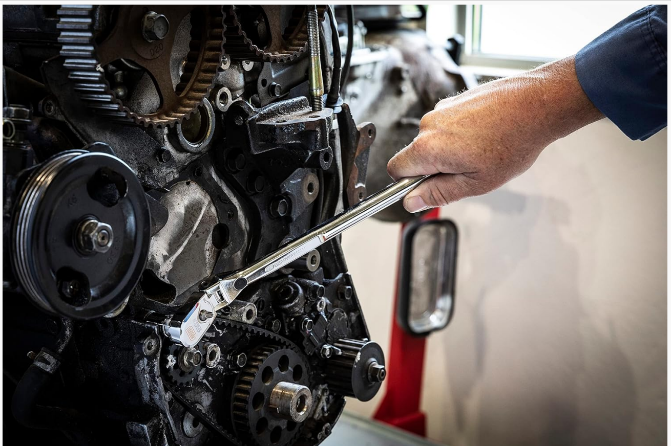
Image 3.1: The longer GEARWRENCH 120XP ratchet being used to access a fastener in an engine compartment, demonstrating the utility of the flexing head.
