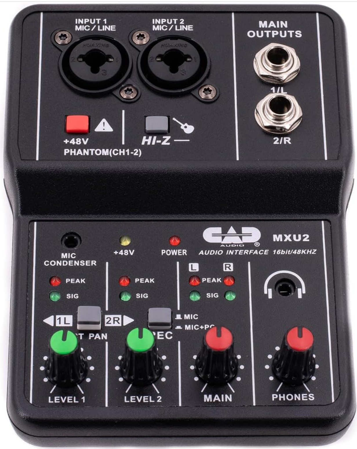
Figure 1: Top-down view of the CAD Audio MXU2 mixer, showing all controls and inputs/outputs.
