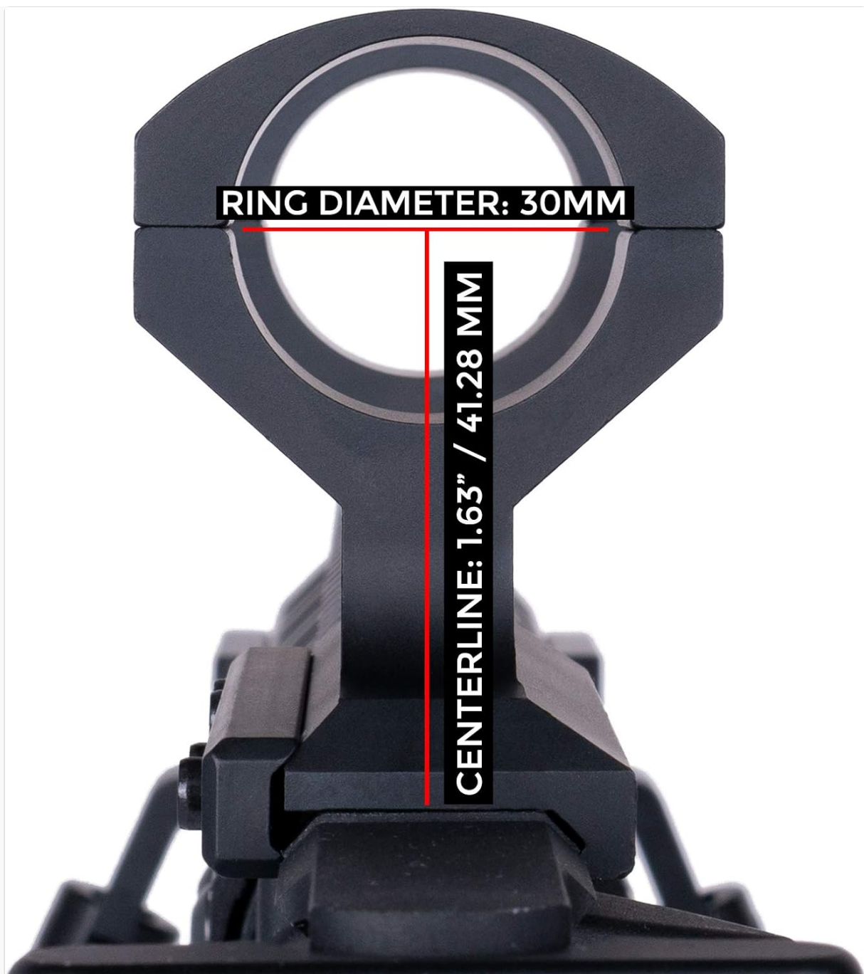
Image 6.3: Front view showing the 30mm ring diameter and 1.63-inch (41.28mm) centerline height of the scope mount.
