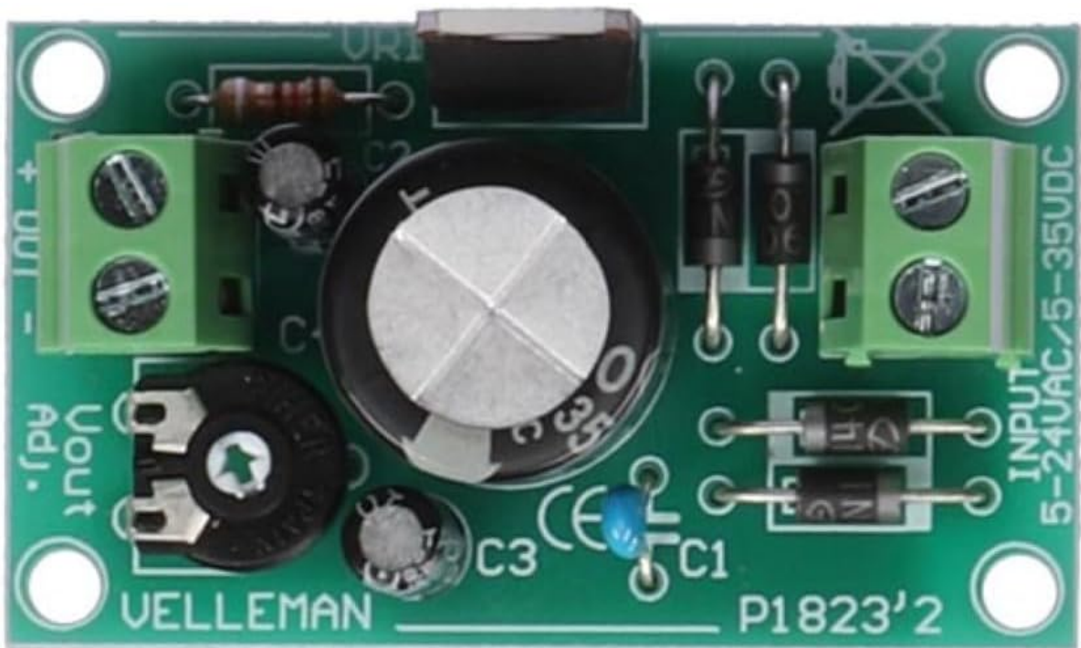
Figure 2: Angled view of the WMPC124 module, showing component layout.
