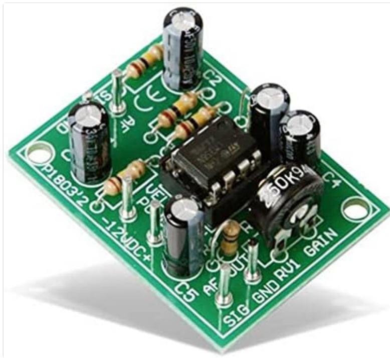
Image: A fully assembled Whadda WSAH1803 Universal Mono Preamplifier circuit board, with all components soldered and the IC inserted into its socket.
