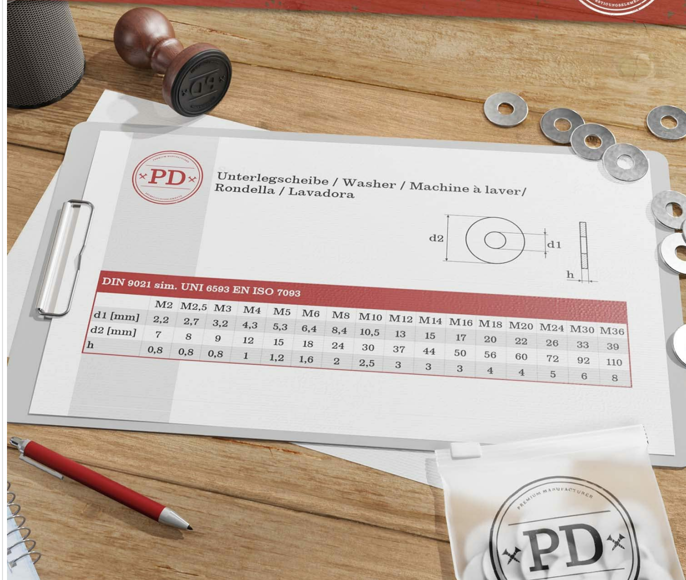
Image: Technical drawing illustrating the dimensions of a washer (d1, d2, h) and a table with various sizes.
