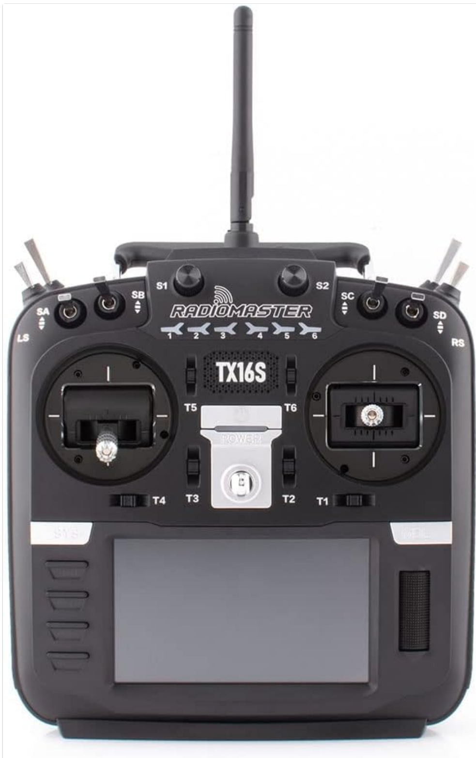
Figure 2.2: Front view of the RadioMaster TX16S MKII V4.0, showcasing the layout of gimbals, switches, and the display area.
