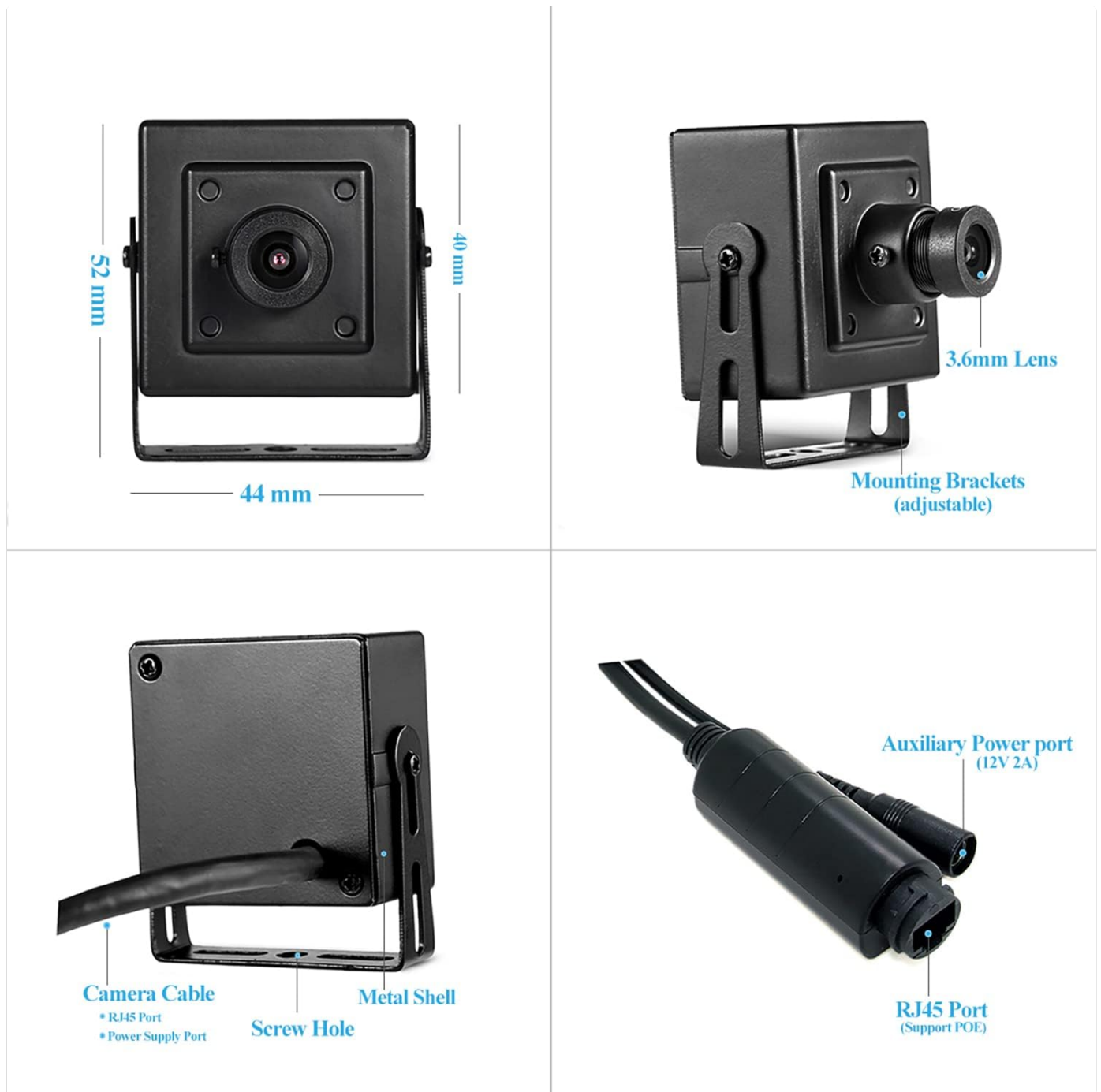
Figure 4: Detailed view of the camera's dimensions, 3.6mm lens, mounting brackets, RJ45 port (for POE), and auxiliary power port (12V 2A).
