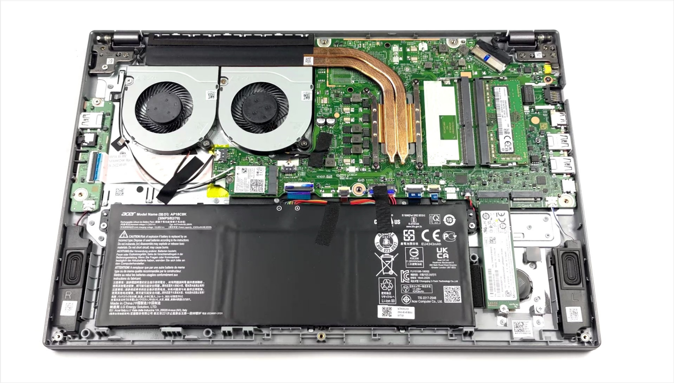
Internal components of the Acer Aspire 5, including the battery, memory slots, and SSD slot.
