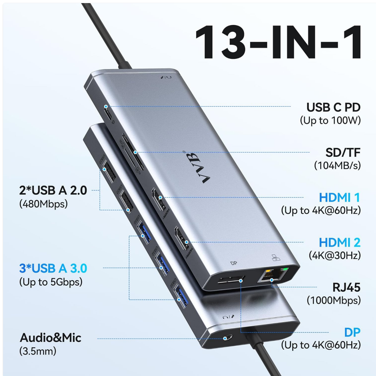
Image 1.1: Front and side view of the VVB 13-IN-1 USB C Hub, illustrating all available ports and their functions.
