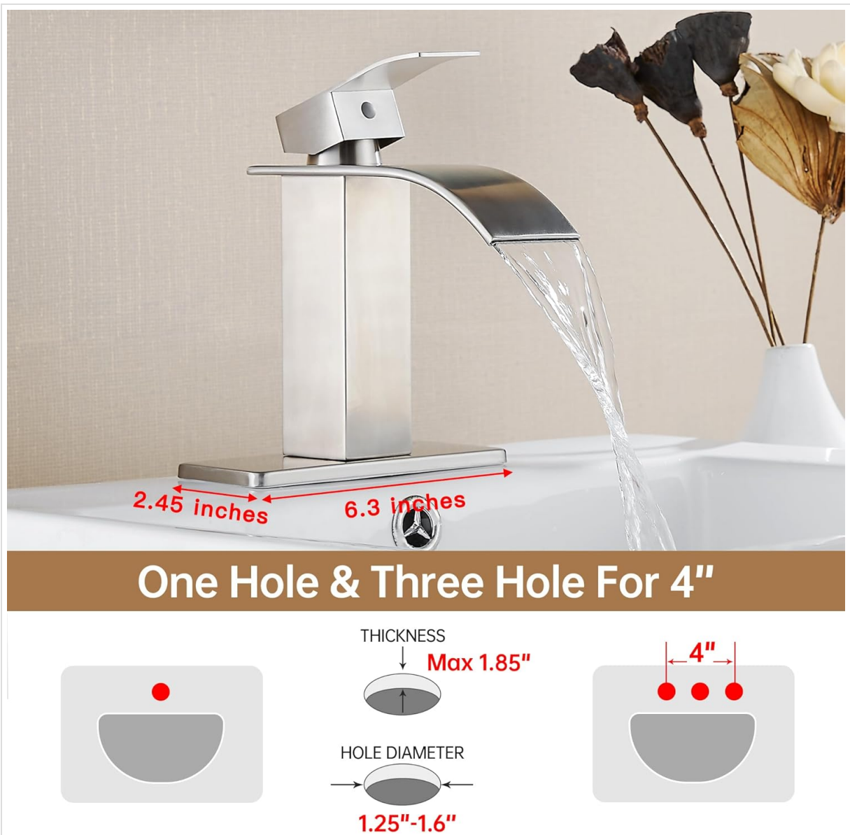
Image: Diagram illustrating the required hole configurations for installation, showing options for single-hole and three-hole sinks with a 4-inch centerset width, along with maximum thickness and hole diameter specifications.
