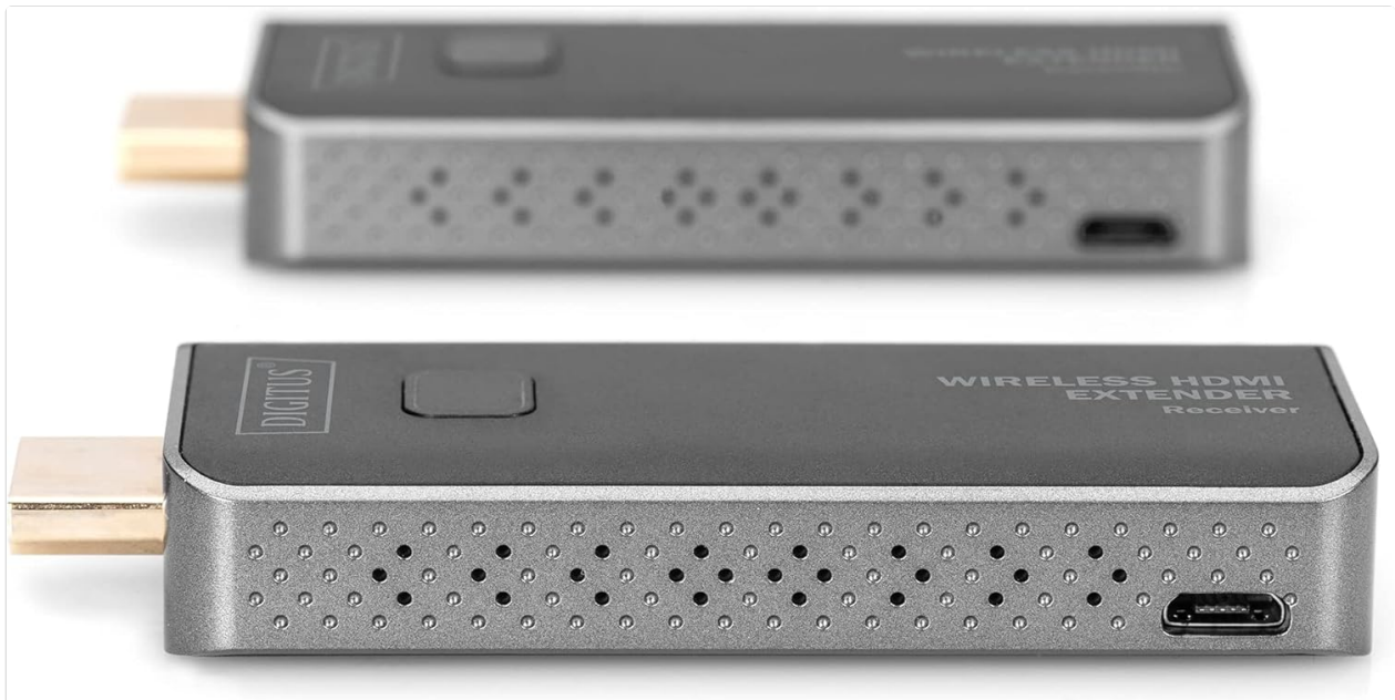
Image 4.3: Side view of the units, showing the Micro-USB power input.
