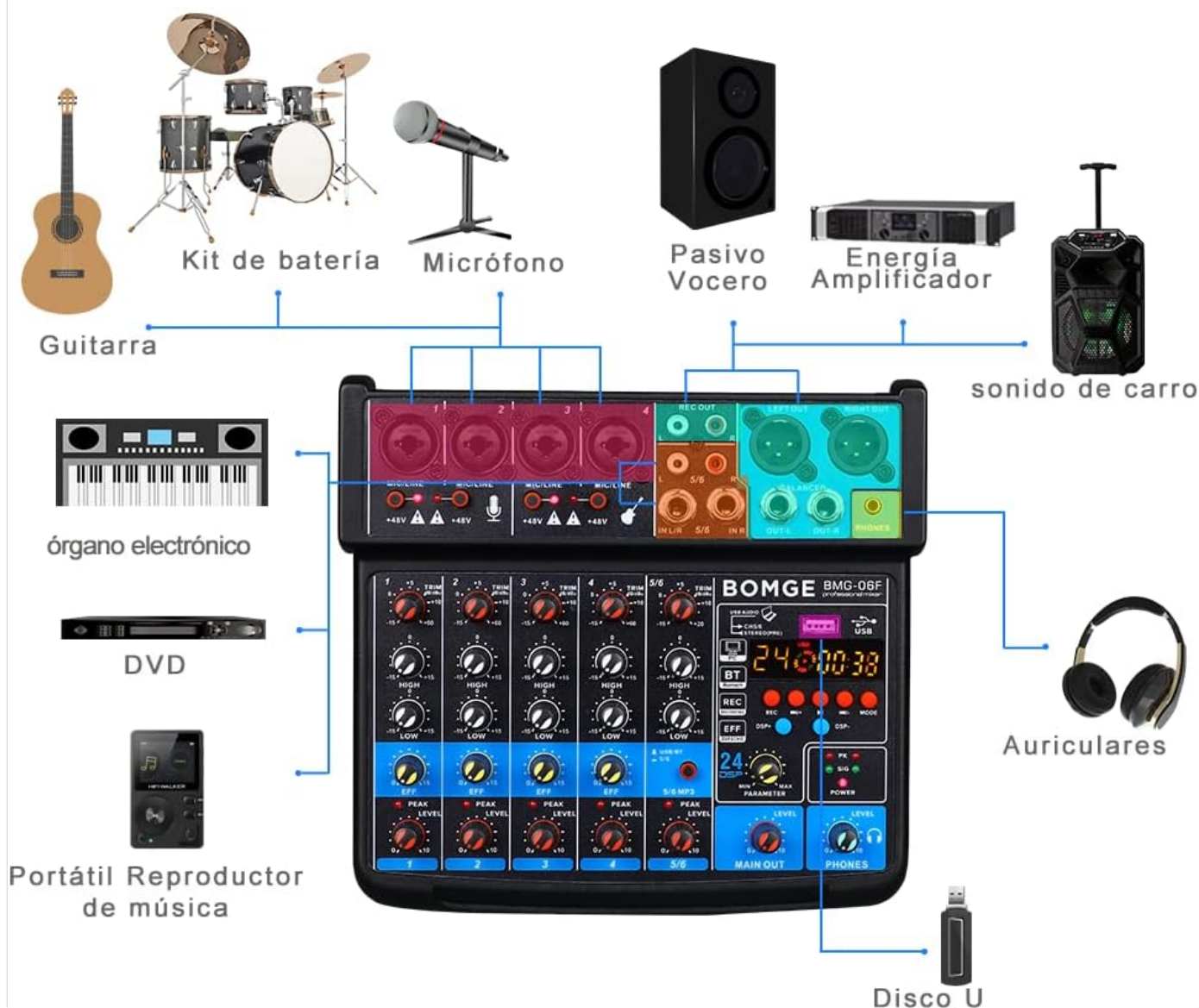
Figure 4.4: Multiple device connection options.
