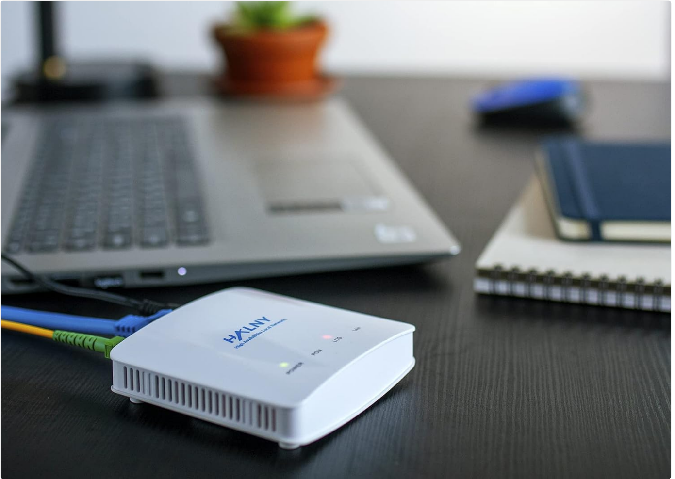
Figure 6.1: The HL-1GE GPON ONT in an operational setup.
