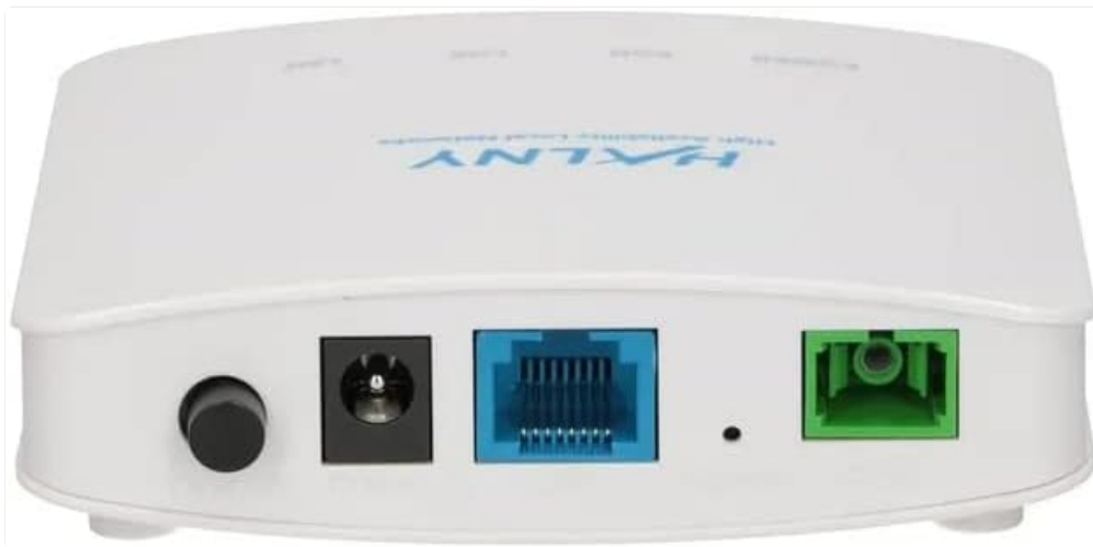
Figure 4.2: Rear view of the HL-1GE GPON ONT, showing the power input, Gigabit Ethernet port, and SC/APC optical port.
