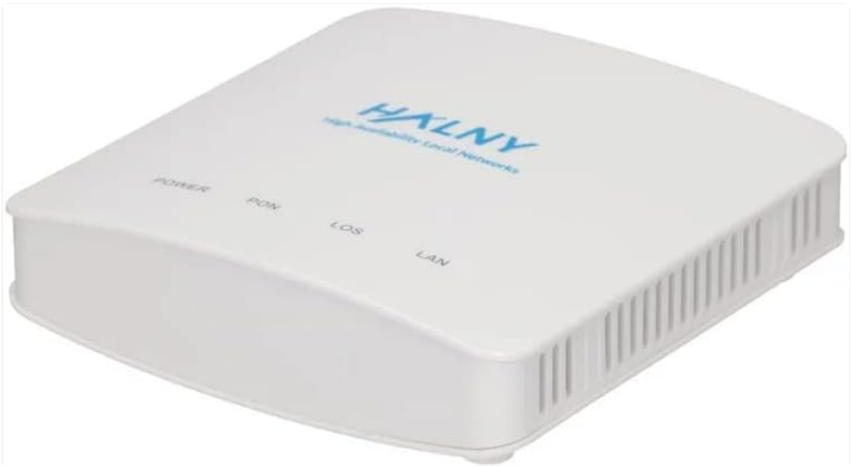
Figure 4.1: Top view of the HL-1GE GPON ONT with LED indicators for Power, PON, LOS, and LAN.
