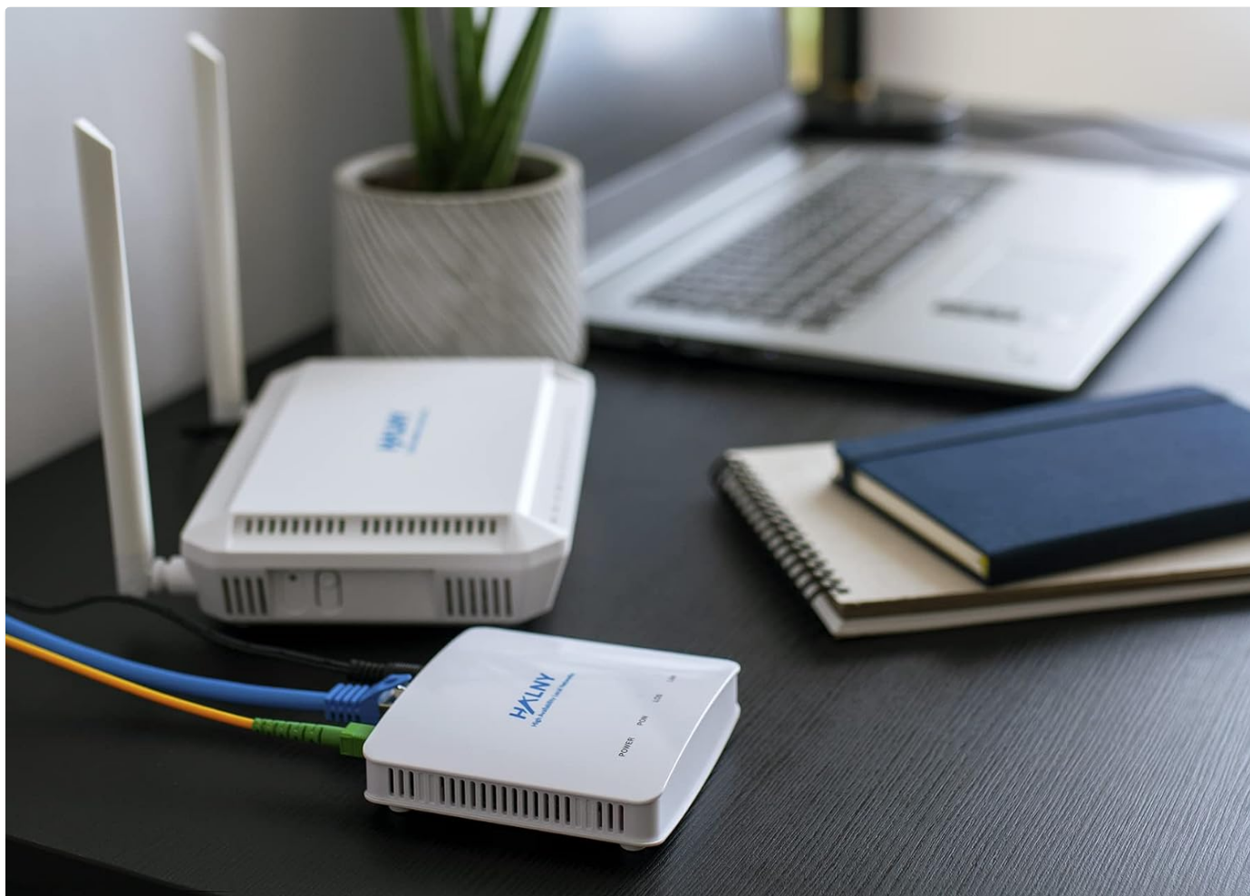
Figure 6.2: The HL-1GE GPON ONT integrated into a network with another router.
