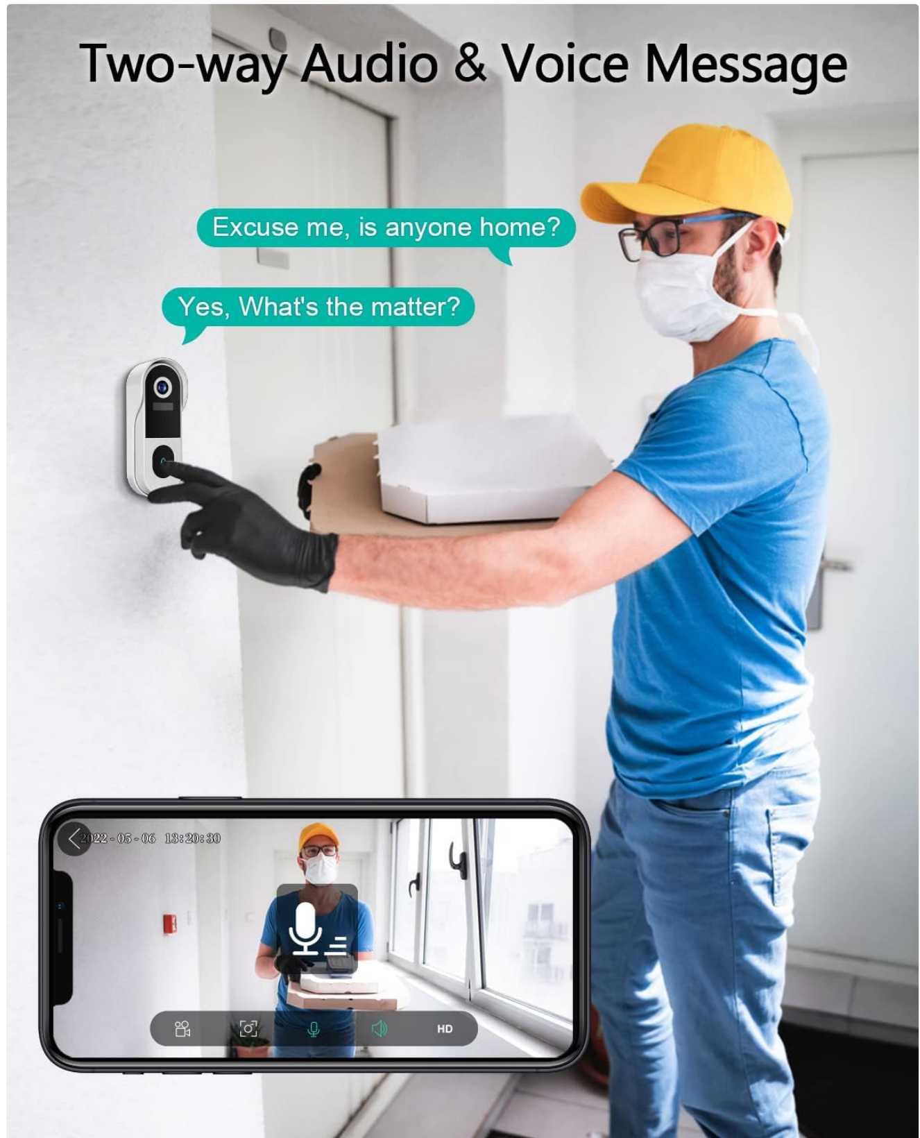
Image 4.1: Demonstrates the two-way audio feature, allowing communication with visitors.
