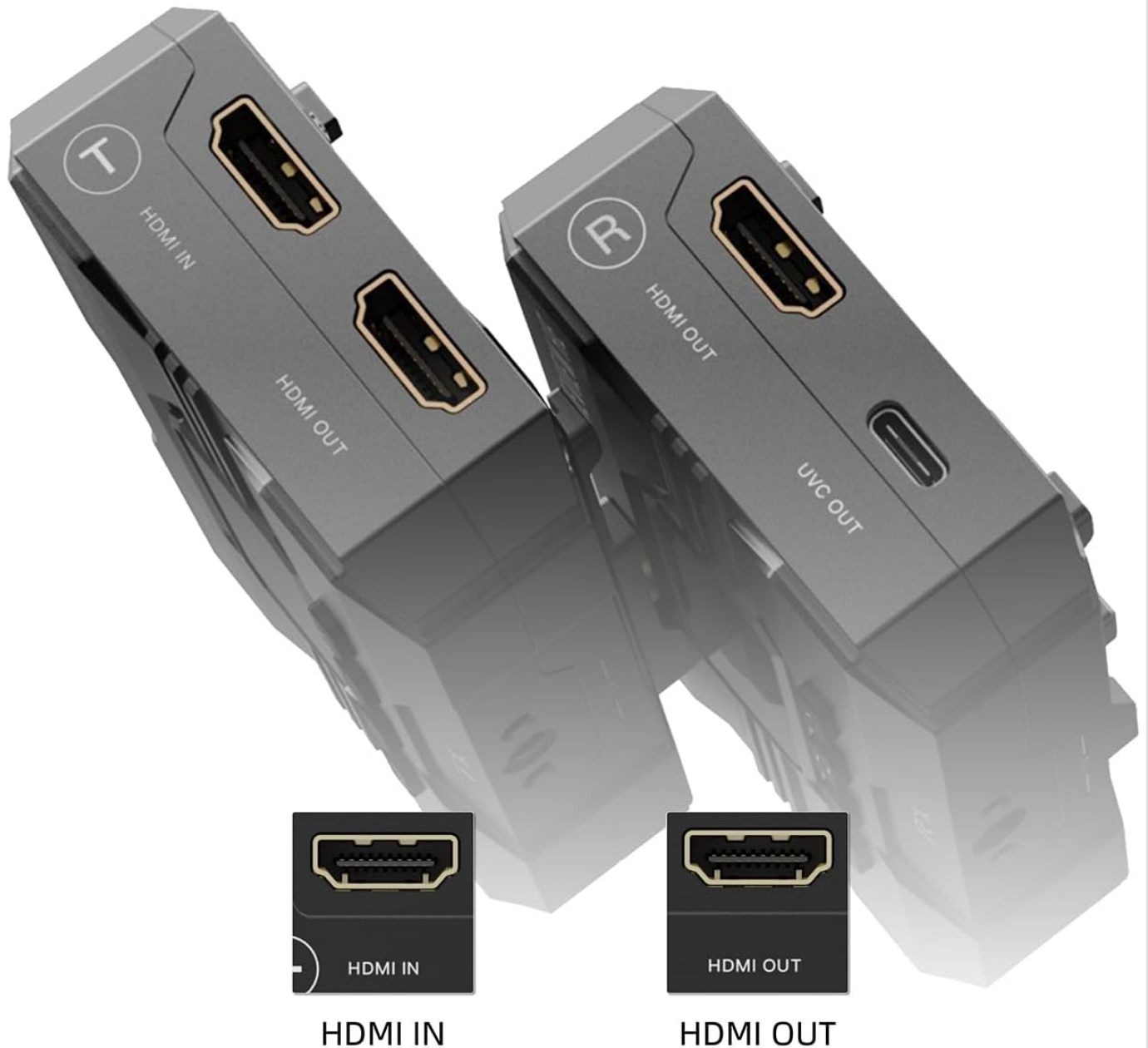
Figure 5.1: Power and HDMI ports on the CineView HE units.
