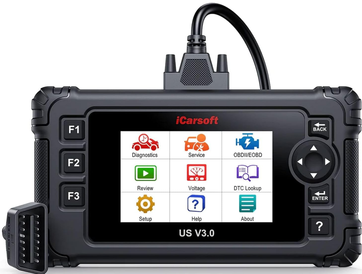
Image: The main menu interface of the iCarsoft US V3.0, displaying various diagnostic and service options.
