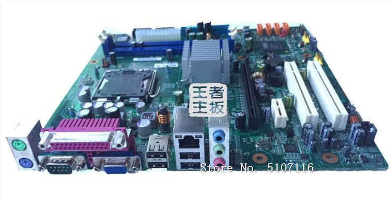
Figure 4.2: Angled view of the BooiParts G31T-LM V1.0 motherboard. This perspective provides a clearer view of the rear I/O panel, including PS/2 ports, serial port, VGA output, USB ports, Ethernet port, and audio jacks. Key components like the chipset heatsink and power delivery components are also visible.
