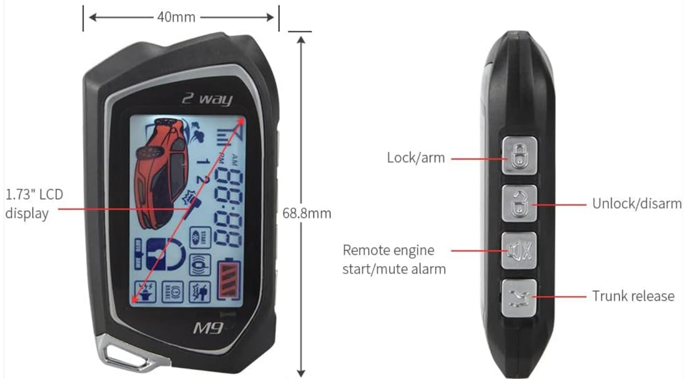
Image: A detailed view of the 2-way LCD remote control, highlighting its 1.73-inch LCD display and labeling the functions of its buttons: Lock/Arm, Unlock/Disarm, Remote Engine Start/Mute Alarm, and Trunk Release.
