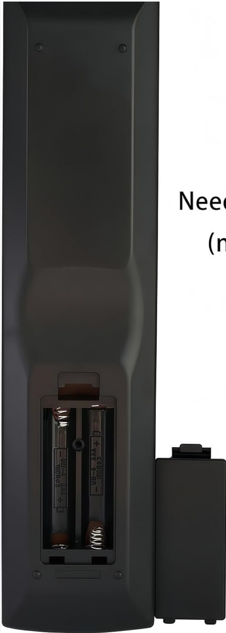
The back of the uehba remote control is shown with the battery cover removed, illustrating the compartment for two AAA batteries.
