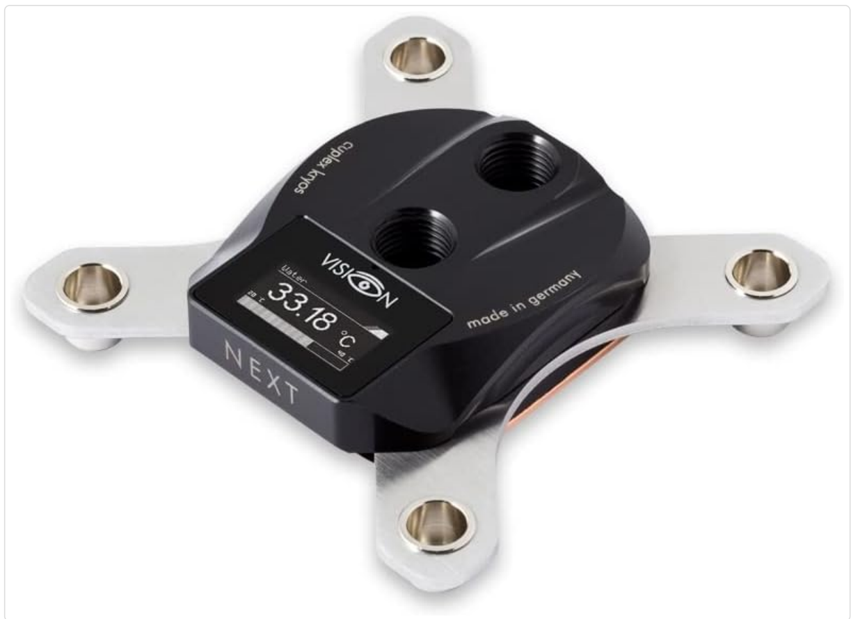
Image 4.1: The Aquacomputer Cuplex Kryos Next with Vision 1700 water block, showing its integrated display and mounting bracket.
