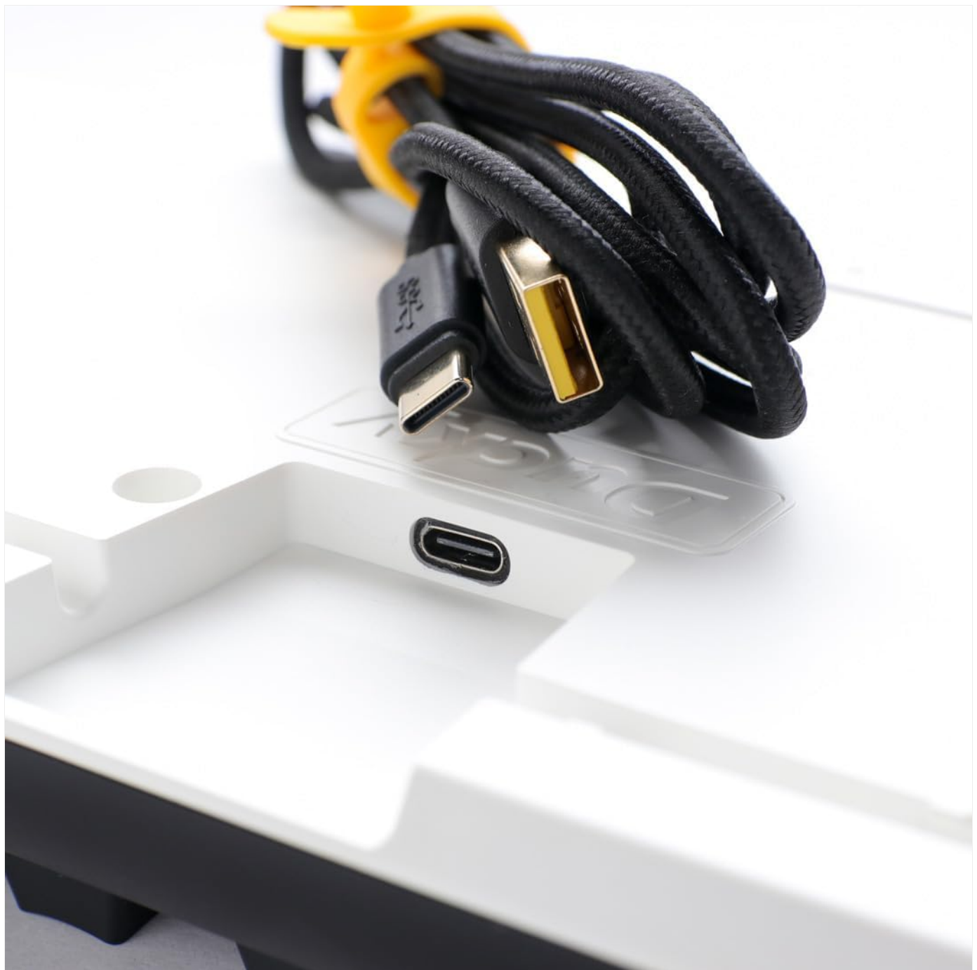
Figure 4: Detail of the detachable USB Type-C port, ensuring reliable and convenient connection.
