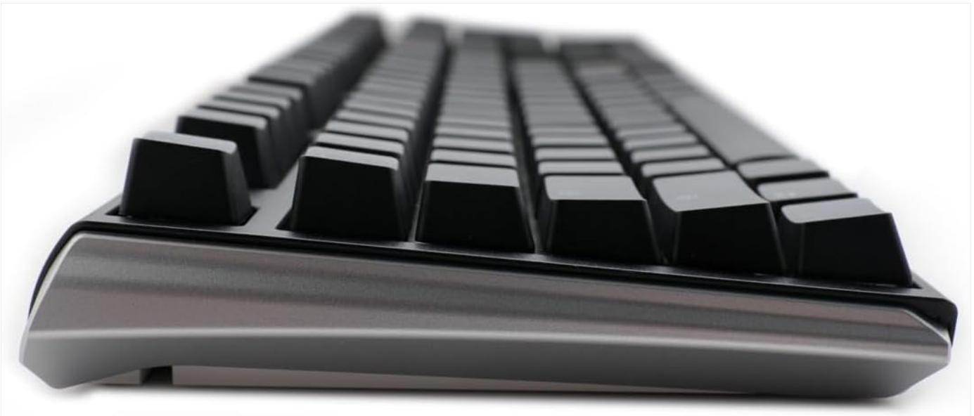
Figure 2: Side view illustrating the low-profile case design of the Ducky One 3 Classic keyboard.
