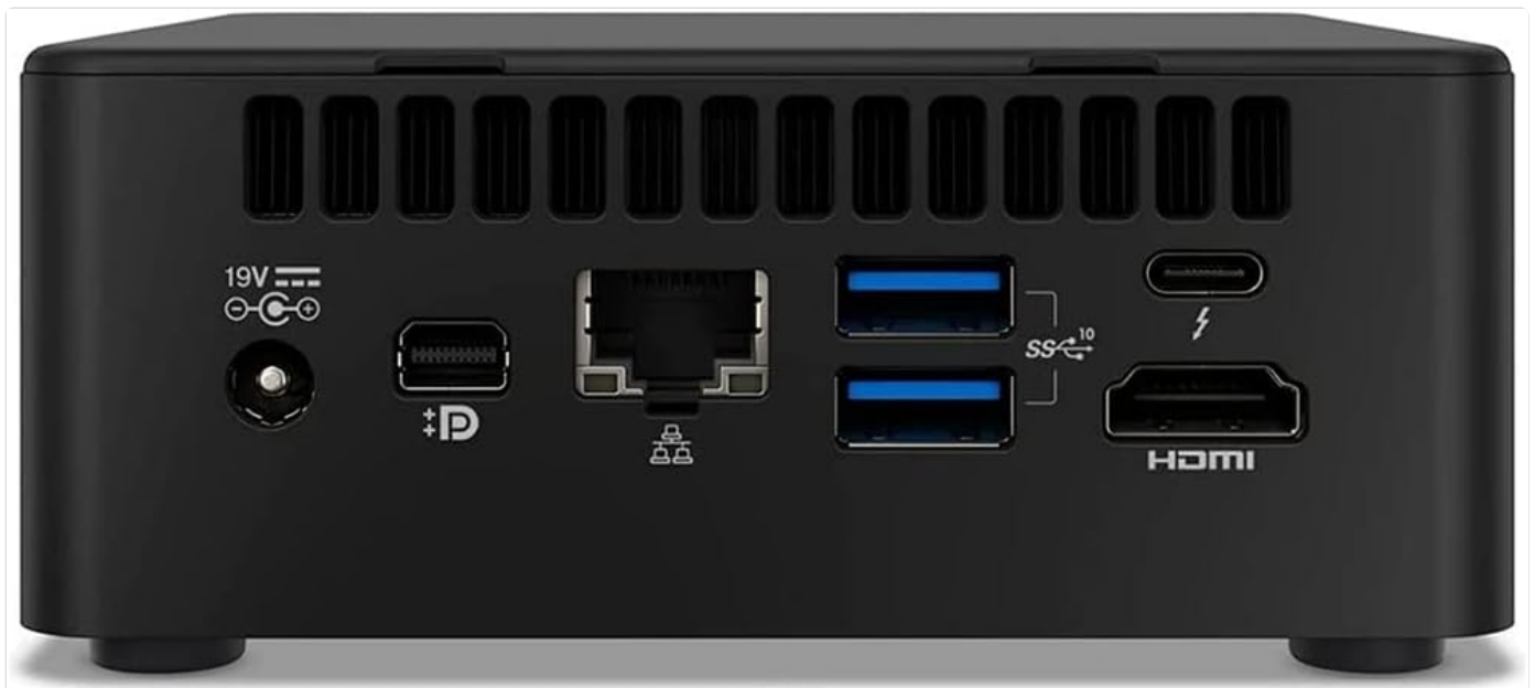
Figure 4.2: Rear view of the Intel NUC11PAHi7 Mini Desktop. This image illustrates the rear panel connectivity options. From left to right, it includes the DC power input (19V), a Mini DisplayPort, an Ethernet (RJ-45) port, two USB 3.2 Gen 2 Type-A ports, a Thunderbolt 4 port (USB-C), and an HDMI port. These ports provide comprehensive options for power, display, networking, and peripheral connections.
