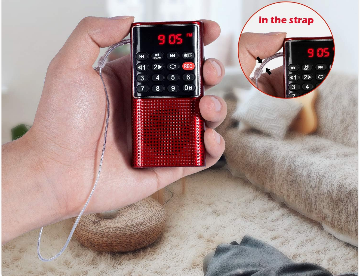
Figure 7: The J-328 radio demonstrating its hidden antenna, integrated into the wrist strap.
