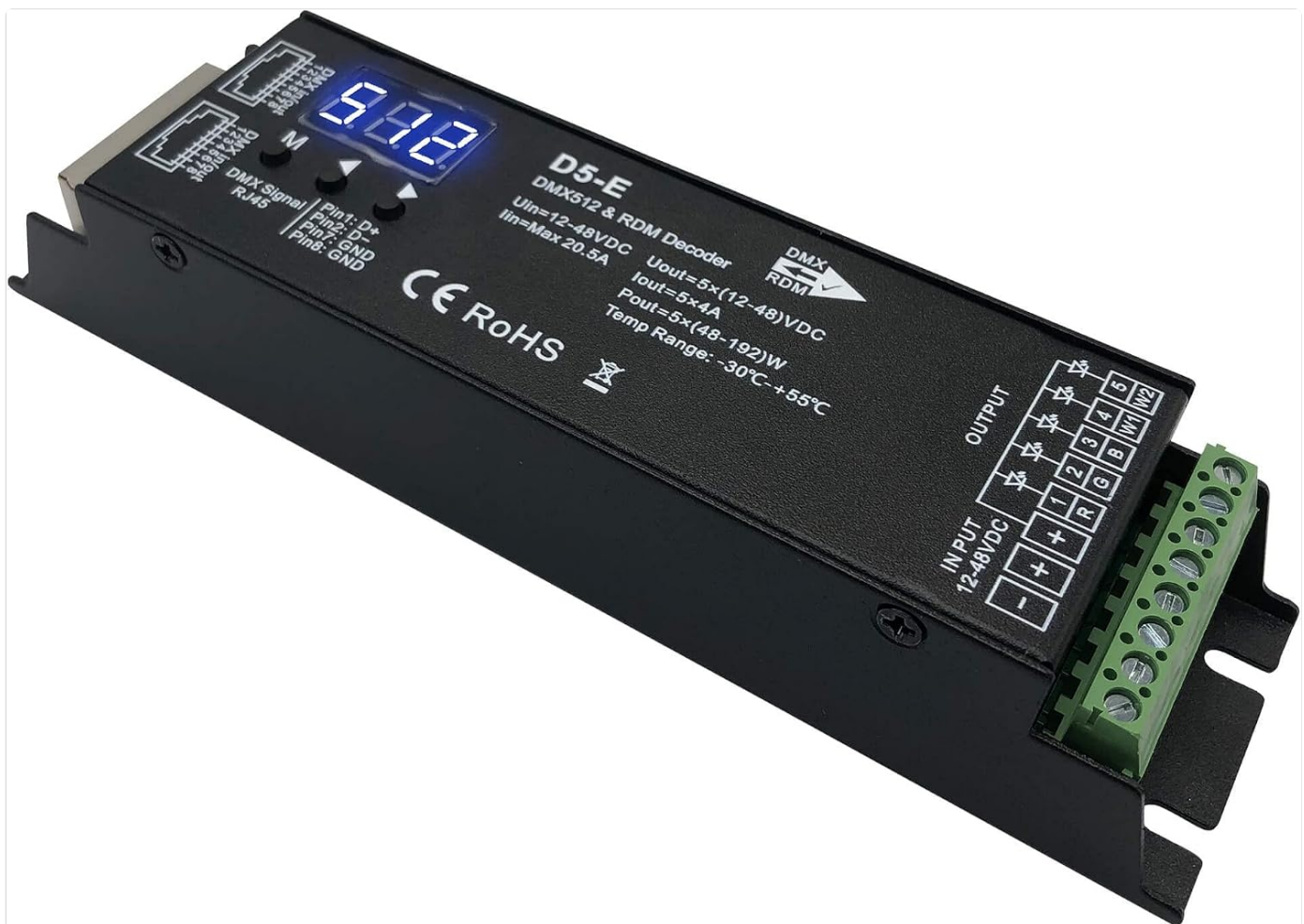
Figure 1: GIDEALED D5-E 5-Channel DMX Decoder
