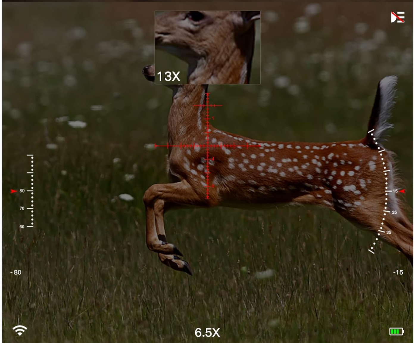
Figure 5: Demonstrates the Picture-in-Picture (PIP) function, showing a magnified view (13x) of the target within the main 6.5x field of view.
