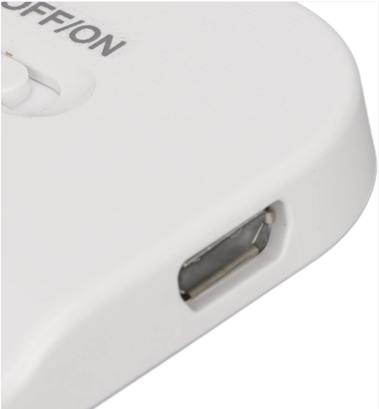
Image: A detailed view of the micro USB charging port on the device.
