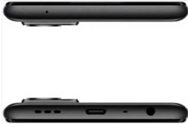
Figure 2.1: Top and bottom views of the OPPO A96, showing the charging port, speaker, and SIM tray location.
