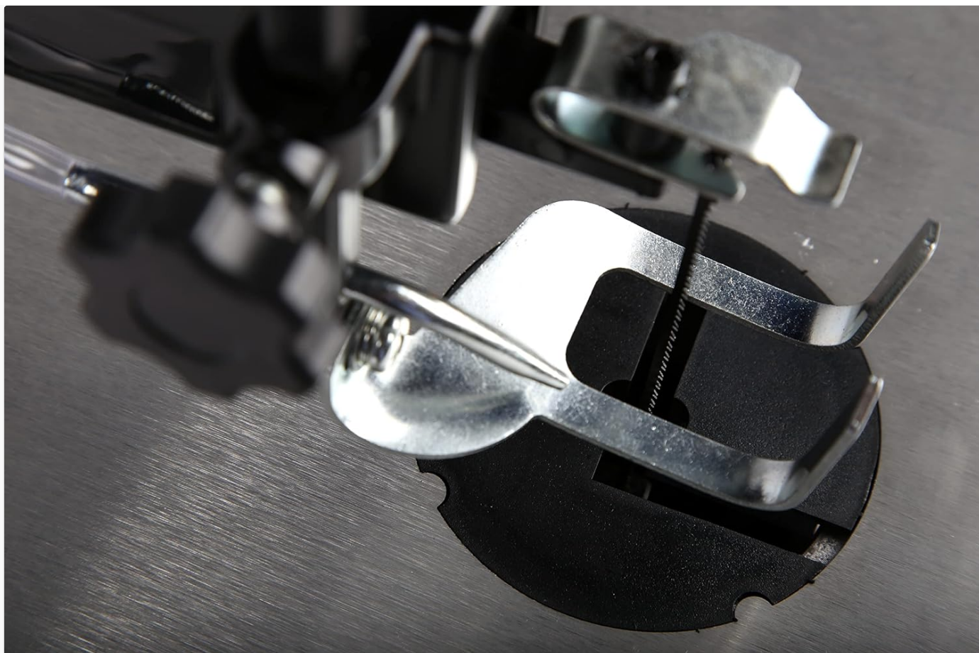
Image: Overhead view of the scroll saw's blade area, showing the blade inserted through the table insert.
