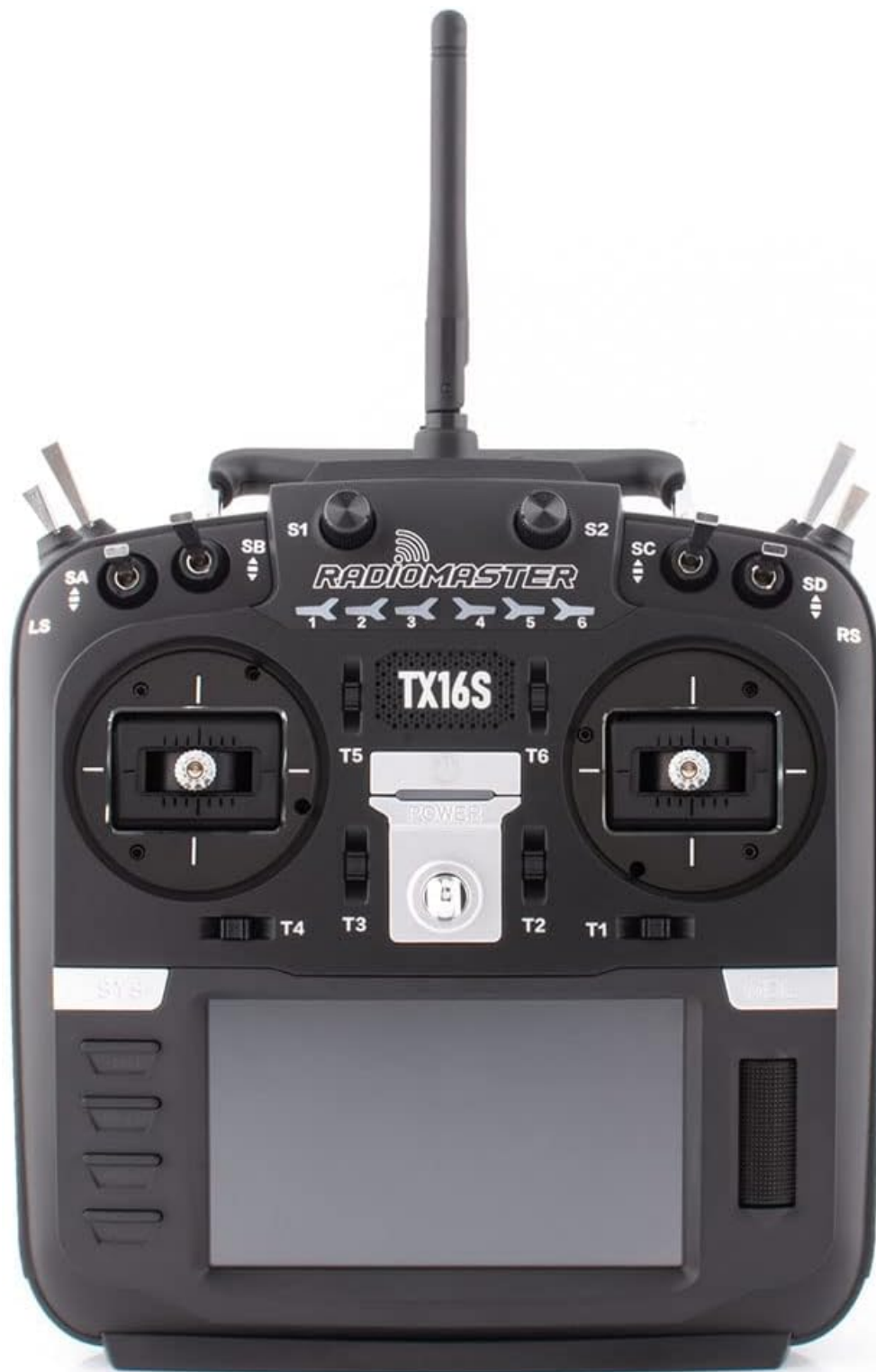
Figure 3.1: Front view of the TX16S Mark II, showing the gimbals, switches, and touchscreen display.
