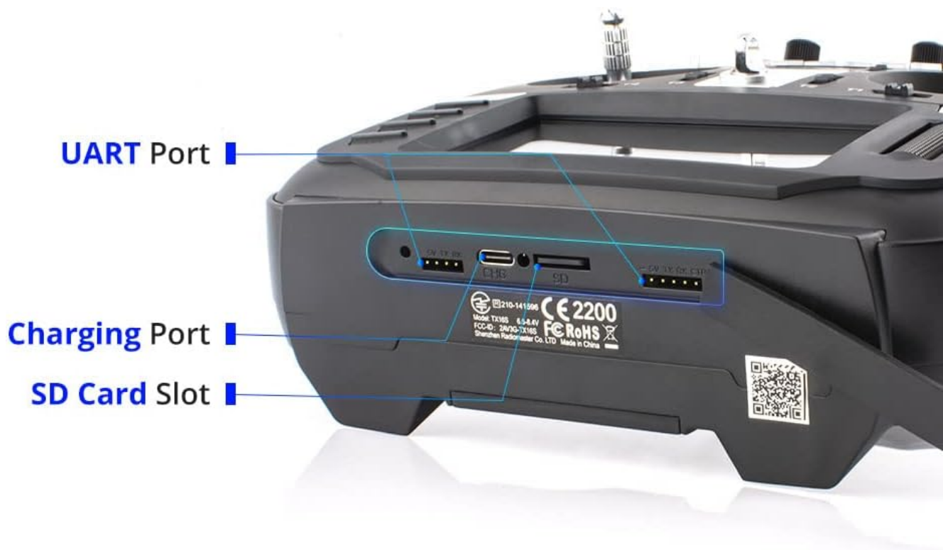
Figure 3.9: Connectivity options include a UART Port, Charging Port (USB-C), and an SD Card Slot for updates and storage.
