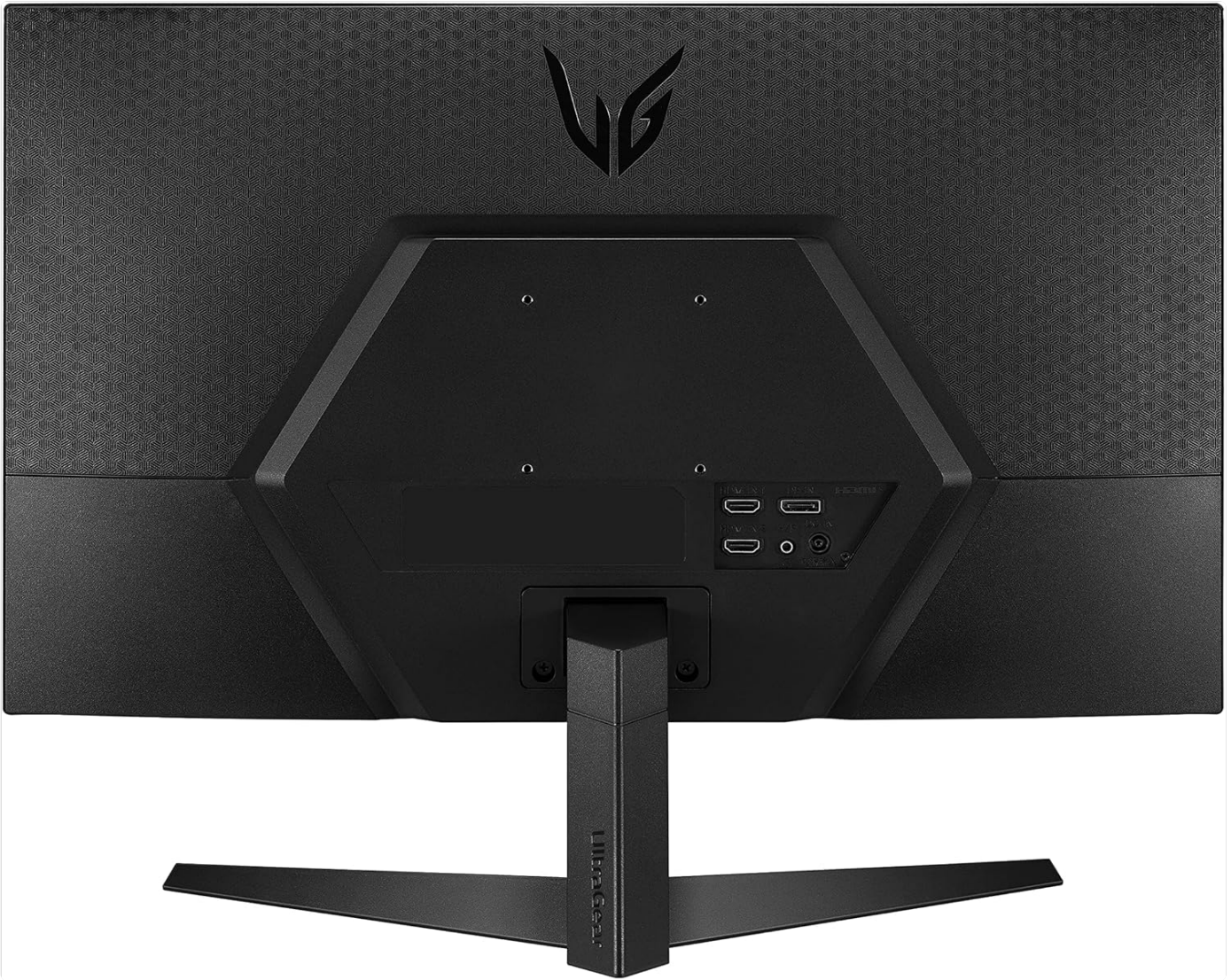
Figure 2.1: Rear view of the monitor showing the stand attachment point and VESA mounting holes.
