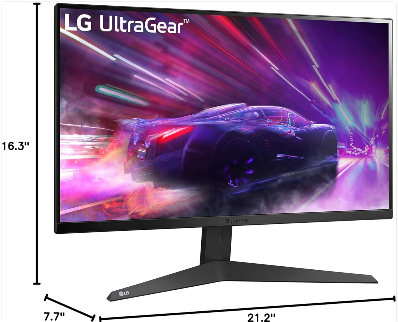
Figure 6.1: Physical dimensions of the LG 24GQ50F-B monitor.
