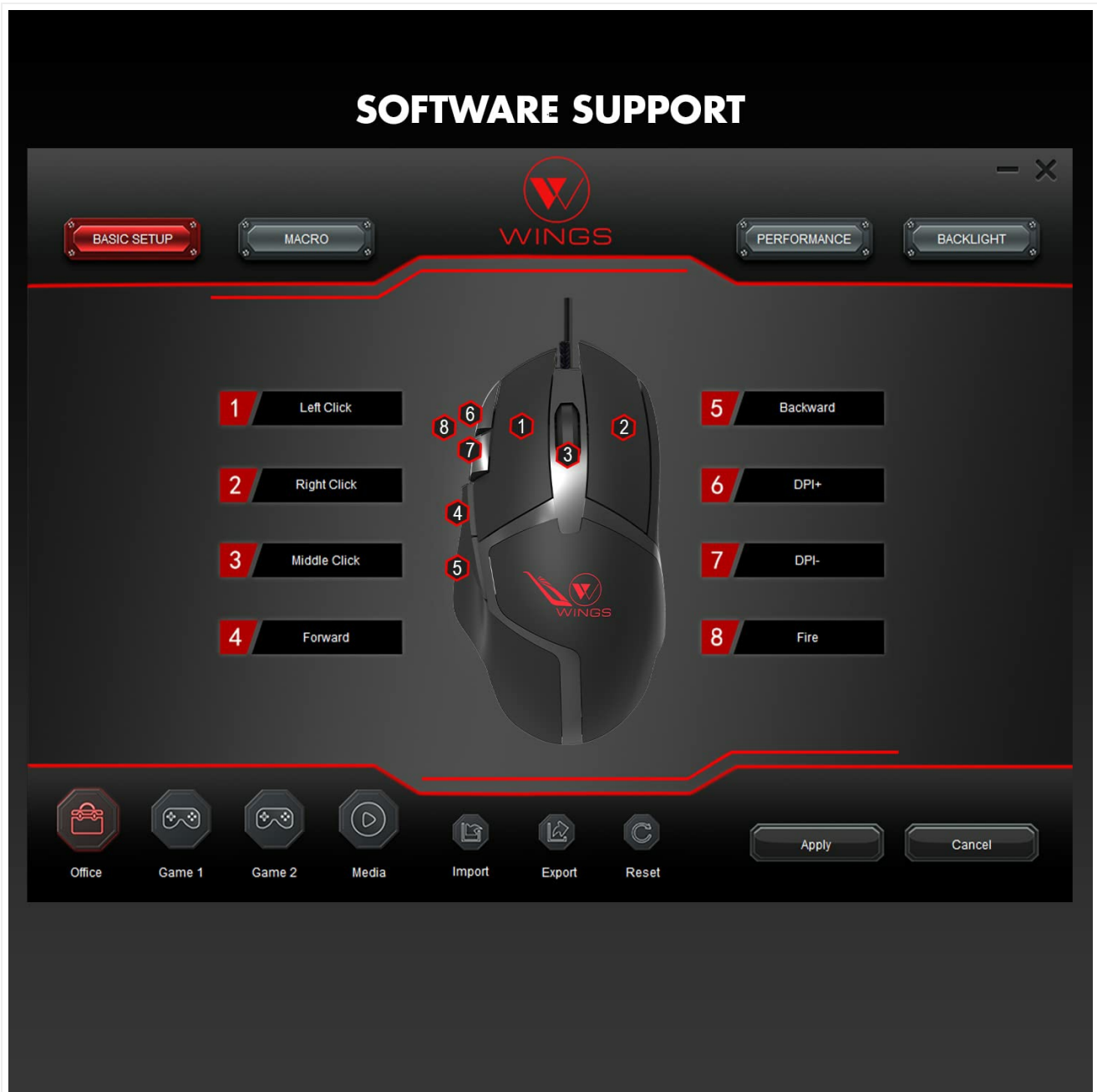
Image 3.2: Example of button assignments within the mouse software.
