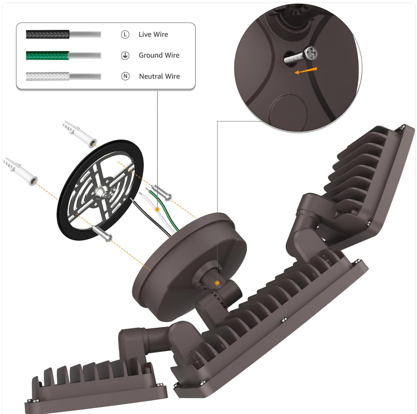
Figure 4: Detailed installation diagram, illustrating the wiring and mounting process.
