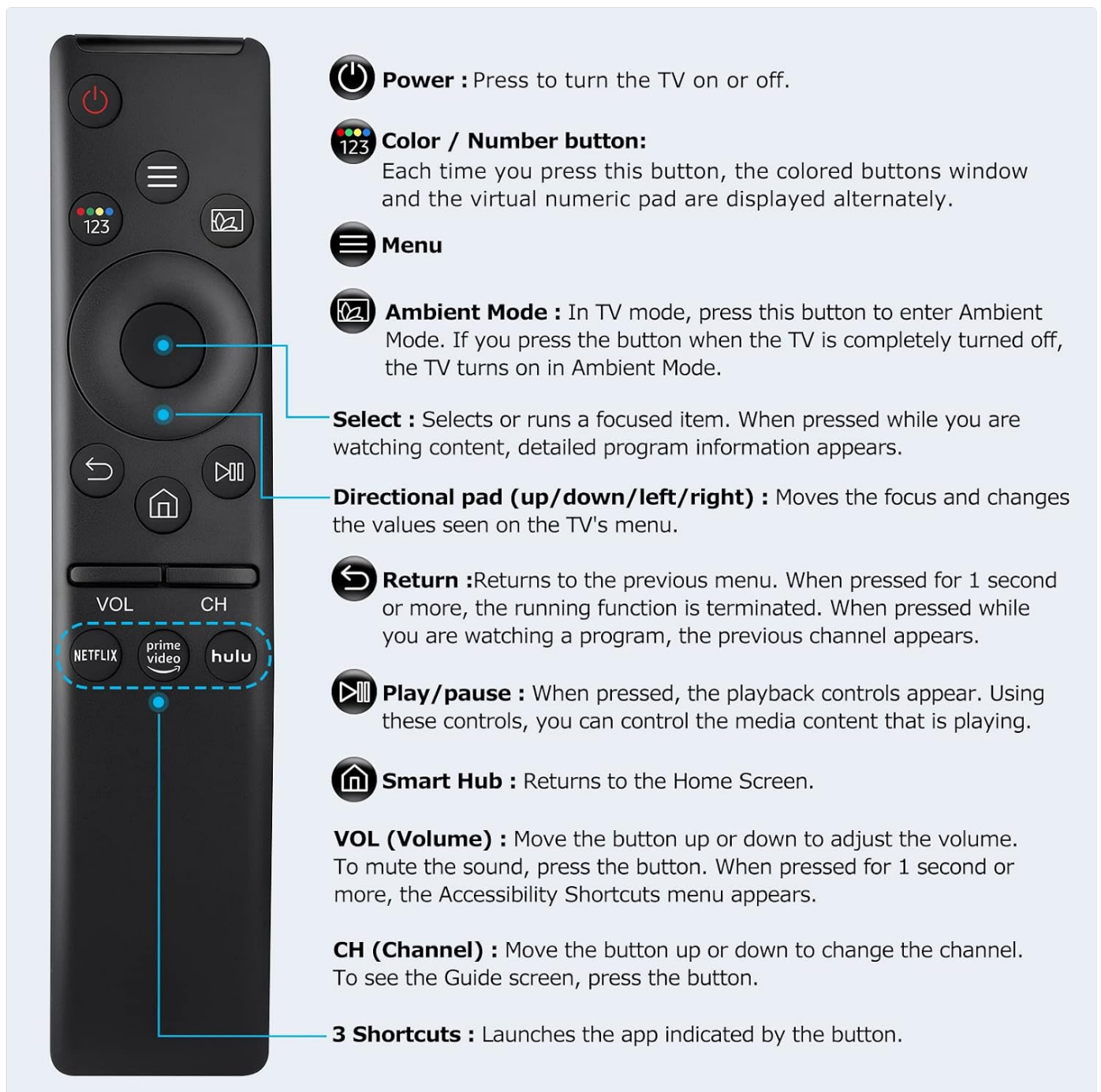
Image: A detailed diagram illustrating the layout of the remote control and the function of each button.
