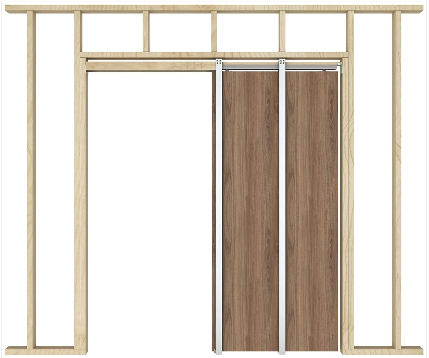
Figure 3: Illustration of a framed wall opening, showing the space required for a pocket door installation.
