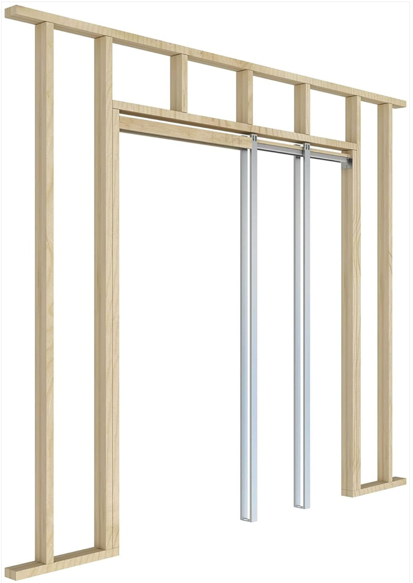
Figure 4: The header assembly, including the aluminum track and wood slot, installed within the rough opening.
