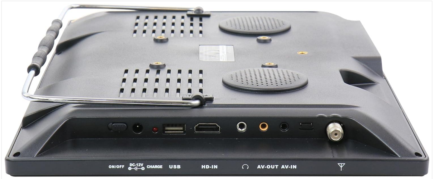
Figure 5: Side panel of the TV, showing the power input, USB port, HDMI input, headphone jack, AV In/Out ports, and antenna input.
